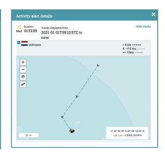
Skylight uses a **machine learning model** based on a database of expert-annotated examples to look for rendezvous behavior in incoming AIS tracks. A Dark Rendezvous event does not guarantee that a rendezvous with a non-AIS transmitting vessel occurred. It just means that the tracks are **exhibiting** characteristic behavior (e.g. slow speeds).
